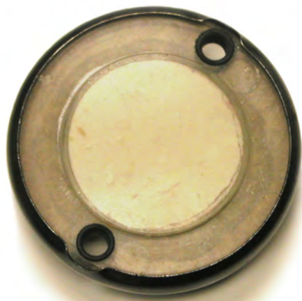
Radioluminescent Deck Marker. Courtesy of Oak Ridge Associated Universities Health Physics Historical Instrumentation Museum Collection.
